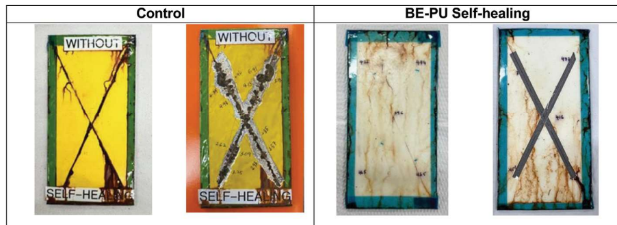
FIGURE 5 Condition of control and BE-PU self-healing specimens after 3,000 h of long-term salt spray exposure testing.
